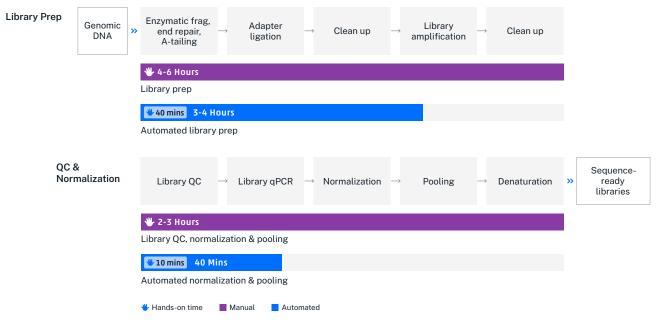
Figure 2. Automating the QIAseq FX and QIAseq Normalizer workflows on the Opentrons Flex reduces total workflow time by several hours and reduces hands-on time to less than one hour. Timings are approximate for 96-sample throughput.
