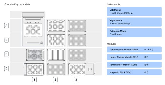
Figure 1. Starting deck layout for a QIAseq workflow on the Opentrons Flex NGS Workstation configured with two Flex 8-Channel Pipettes, Flex gripper and on-deck modules.
