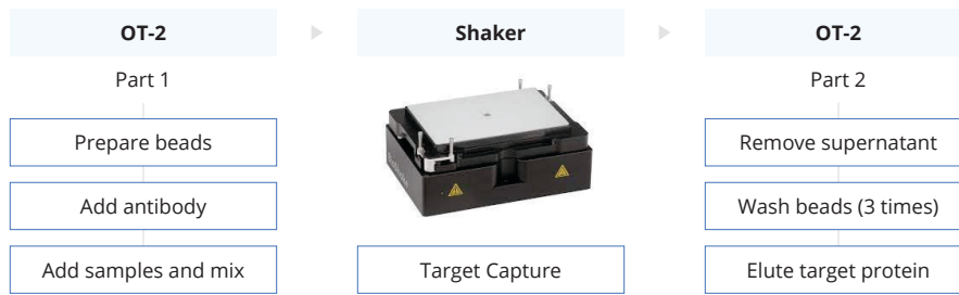
Figure 1: This is an overview of the 3 major steps of protein purification on the OT-2.
