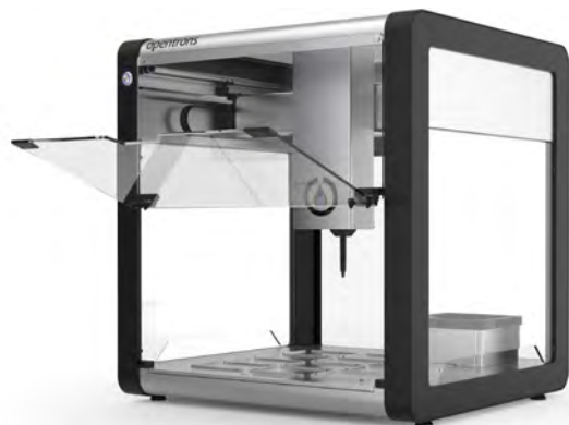
Figure 1: The Opentrons OT-2 is equipped with the Opentrons Magnetic Module and Opentrons GEN2 Pipettes for NGS clean-up. The Magnetic Modules uses high-strength magnetic bars that can be engaged to magnetize magnetic beads, and disengaged to allow magnetic beads to remain in solution.
