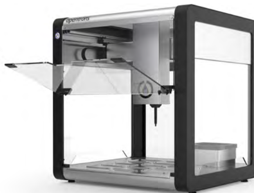
Figure 1: The Opentrons OT-2 is equipped with the Opentrons Magnetic Module and Opentrons GEN2 Pipettes for NGS clean-up. The Magnetic Modules uses high-strength magnetic bars that can be engaged to magnetize magnetic beads, and disengaged to allow magnetic beads to remain in solution.
