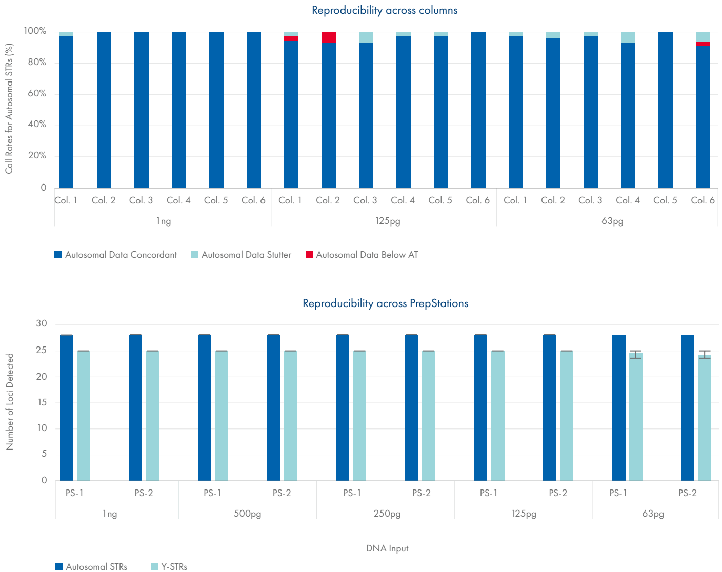
Figure 3. Libraries prepared on the Opentrons Prepstation are highly reproducible across instruments (above) and across columns within the same instrument (below). Autosomal STR data shown.
