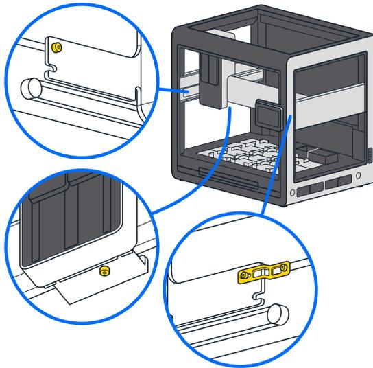
The gantry moves easily by hand after removing all the shipping screws.
