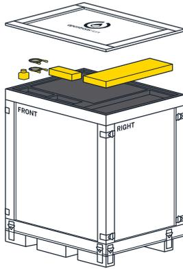
**3** Remove the top piece of foam padding to expose the window panels. Remove the window panels and set them aside. You'll attach these later.
