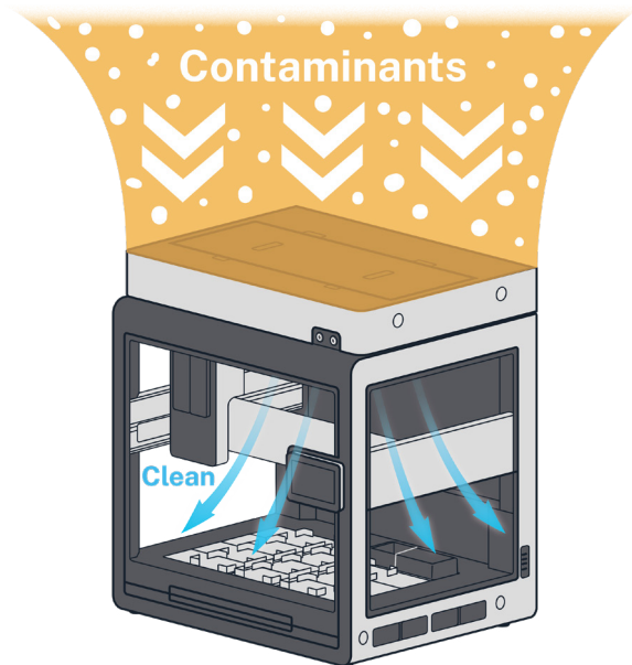
Illustration of contaminants filtered through the HEPA/UV module into the Flex
